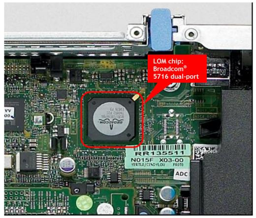
Figure 19. Embedded NICs/LAN on Motherboard
