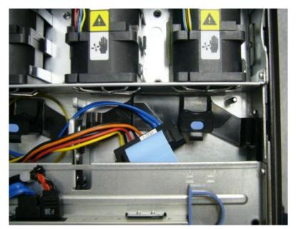
Figure 23. Cabled HDD Connectors
