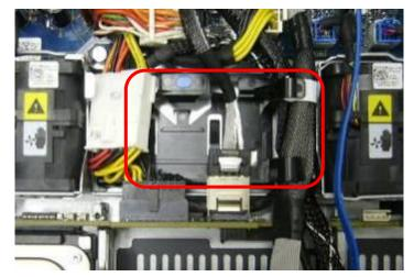
Figure 16. Battery Holder for PERC
