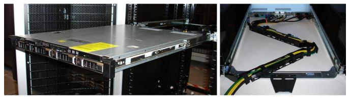
Figure 28. R410 Mounted in the A3 Sliding Rails with the CMA
