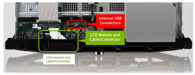
Figure 12. Front Controller Board with LCD
