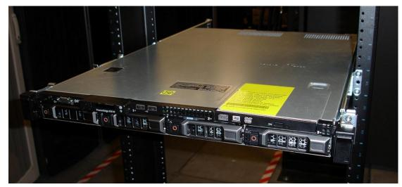
Figure 29. R410 Mounted in the A4 Static Rails in 2-post Center Mount Configuration
