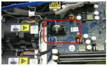
Figure 15. Battery Holder for PERC 6/i
