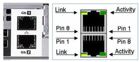
Figure 8. Dual-Stacked RJ45 Connectors with NIC Indicators
