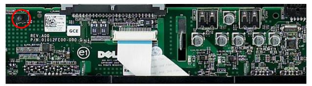
Figure 14. Chassis Intrusion Switch
