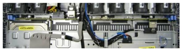
Figure 21. Top-View for Hot-Swap HDD Connection
