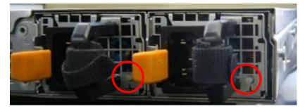
Figure 7. Redundant Power Supply Units
