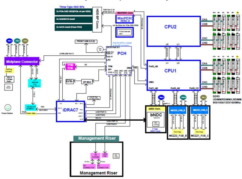
Figure 9. M620 system board block diagram
