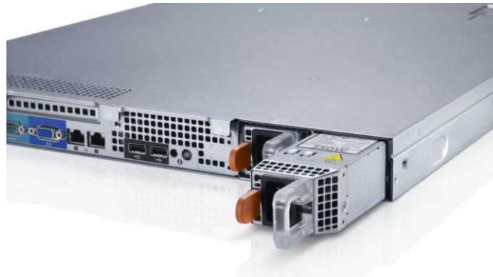
Figure 7. 350W power supply unit
