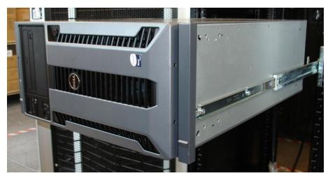
Figure 12. T610 Mounted in C1 Sliding Rails
