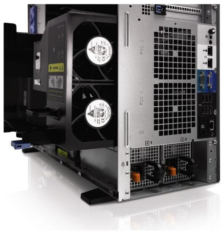
Figure 5. Fans and Cooling Shroud
