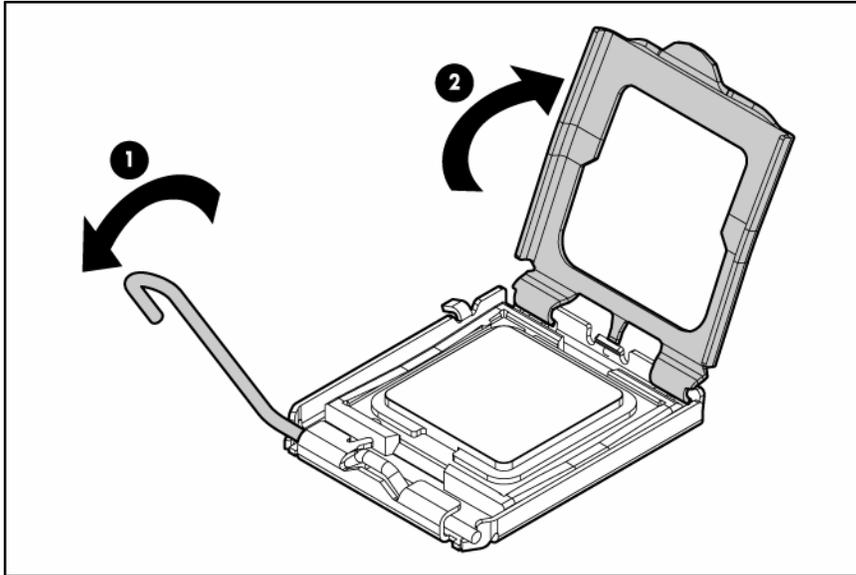
18. Using your fingers, remove the processor from the failed system board.
