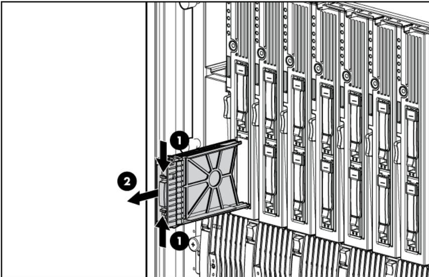
To replace the component, slide the component into the bay until it clicks.
