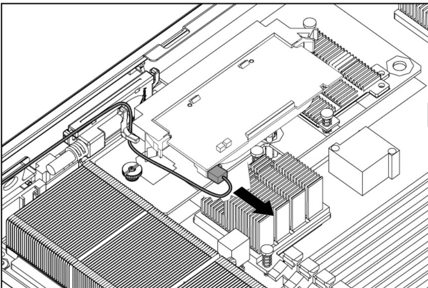
5. Open the flip-top compartment and remove the BBWC carrier from the keyholes.
