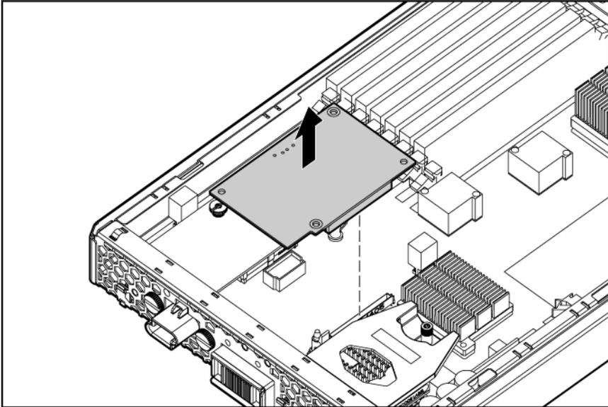
To install the component, reverse the procedure, and be sure to align the FC mezzanine with the FC connectors ("Internal components" on page 56).
