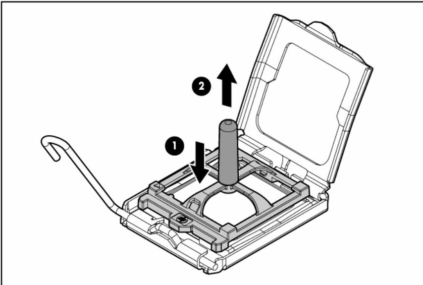
10. Close the processor retaining latch and the processor socket retaining bracket.
