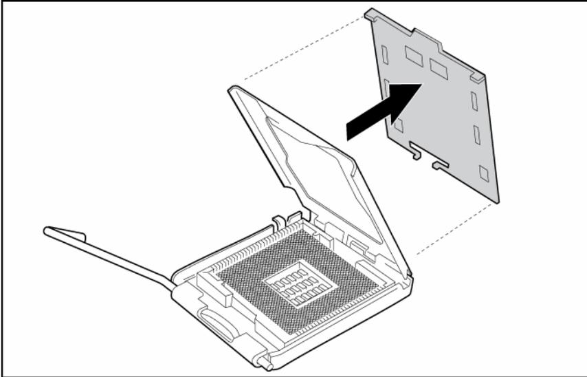
3. Install the processor socket cover onto the processor socket of the failed system board. The cover protects the socket during shipping when the failed board is returned.
