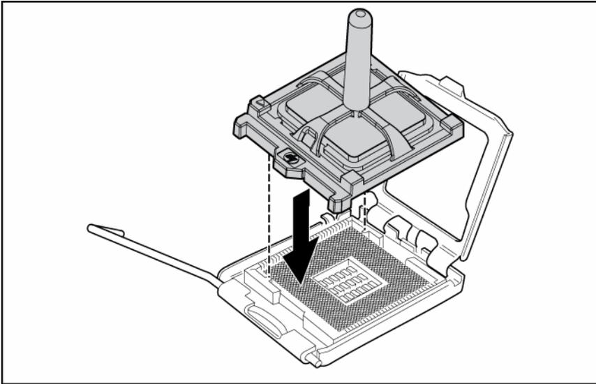
9. Press down firmly until the processor installation tool clicks and separates from the processor, and then remove the processor installation tool.
