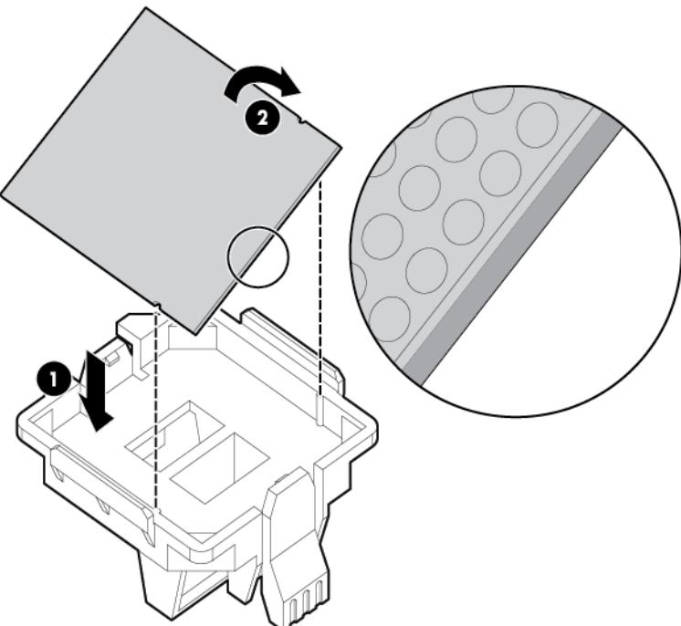
2. Be sure the tool is oriented correctly. Align the processor installation tool with the socket, and then install the processor. **THE PINS ON THE SYSTEM BOARD ARE VERY FRAGILE AND EASILY DAMAGED.**
