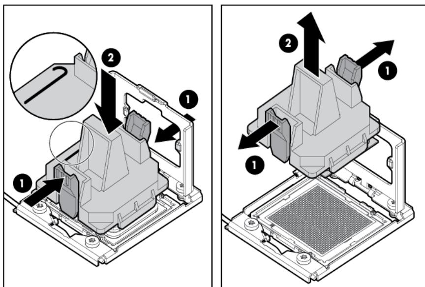
12. Carefully rotate the tool, and then push in and release the tabs to secure the processor in the tool.
