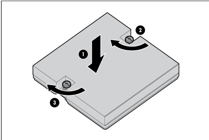
4. Install the front panel/hard drive cage assembly ("Front panel/hard drive cage assembly" on page 33).
