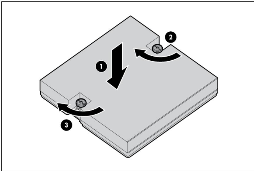
8. Install the front panel/hard drive cage assembly ("Front panel/hard drive cage assembly" on page 33).
