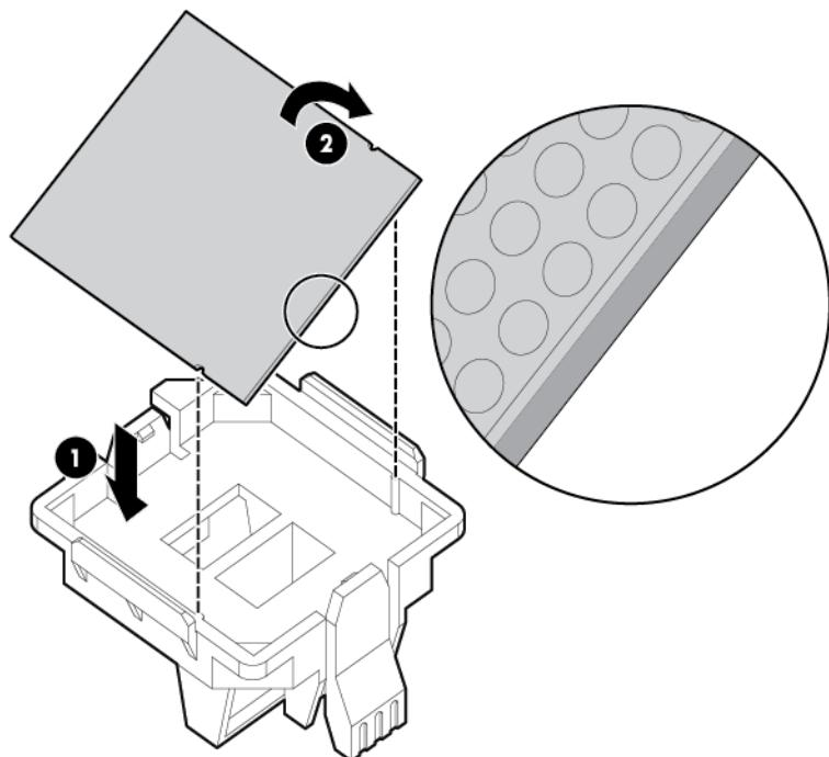
4. Align the processor installation tool with the socket, and then install the processor. **THE PINS ON THE SYSTEM BOARD ARE VERY FRAGILE AND EASILY DAMAGED.**
