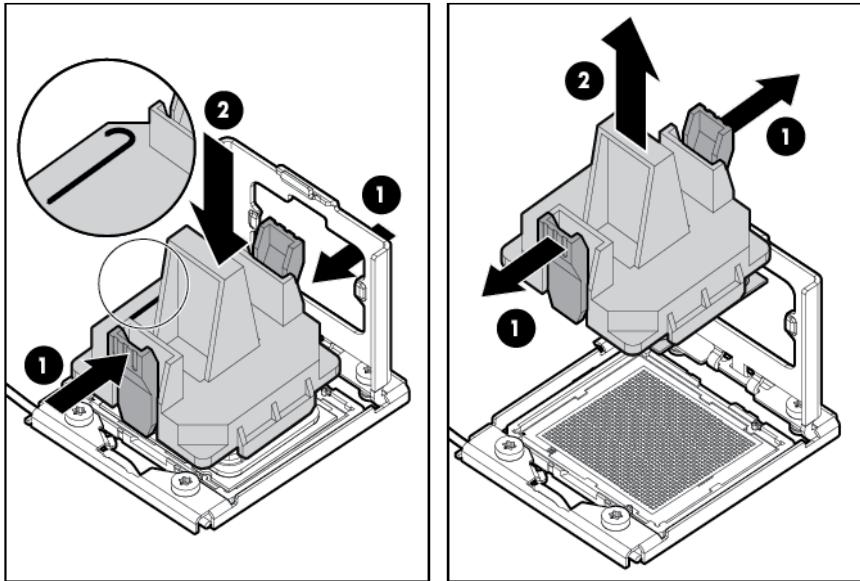
13. Carefully rotate the tool, and then push in and release the tabs to secure the processor in the tool.
