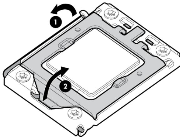
11. Using the processor tool, remove the processor from the system board:
