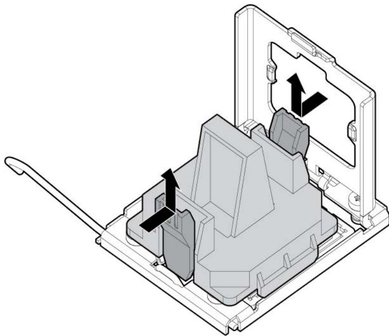
6. Close the processor socket retaining bracket and the processor locking lever. **The processor socket cover is automatically ejected**. Remove the cover.
