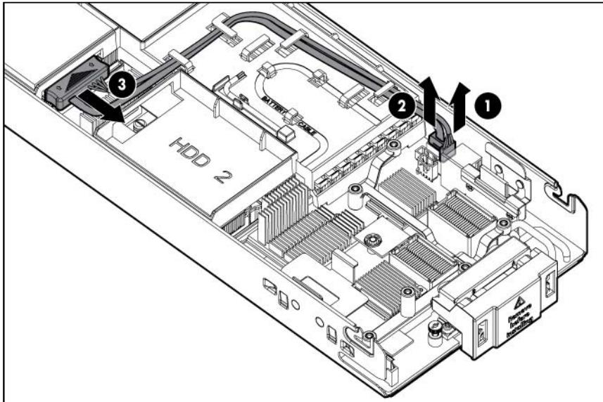
5. Remove the DIMM baffle.
