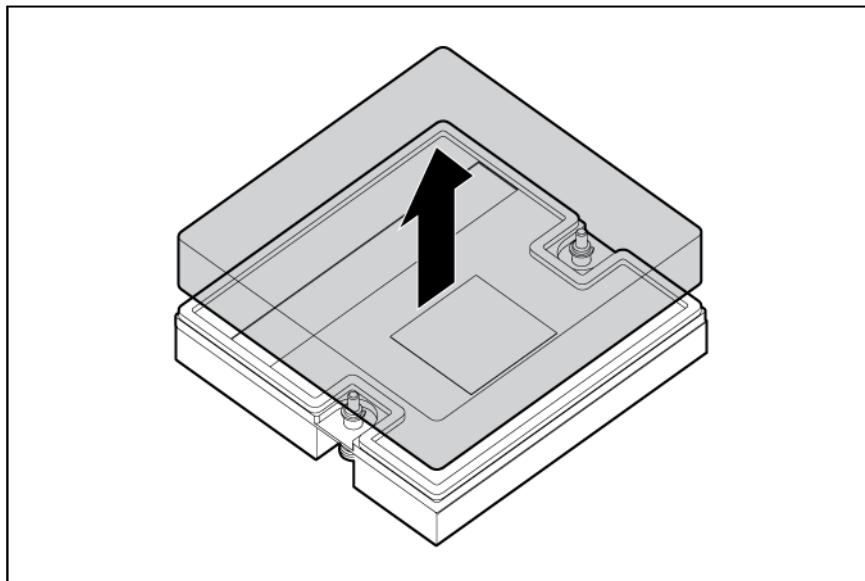
**△ CAUTION:** To avoid damage to the system board, processor socket, and screws, do not overtighten the heatsink screws. Use the wrench supplied with the system to reduce the possibility of overtightening the screws.
