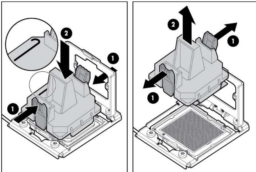
9. Carefully rotate the tool, and then push in and release the tabs to secure the processor in the tool.
