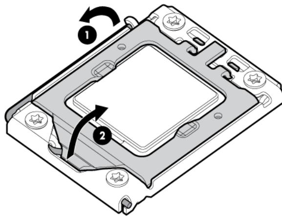
8. Using the processor tool, remove the processor from the system board:
