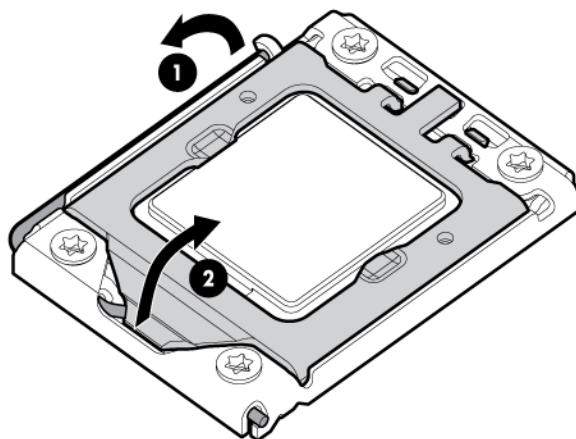
12. Using the processor tool, remove the processor from the system board:
