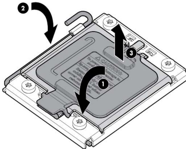
**CAUTION:** Be sure to close the processor socket retaining bracket before closing the processor locking lever. The lever should close without resistance. Forcing the lever closed can damage the processor and socket, requiring system board replacement.
