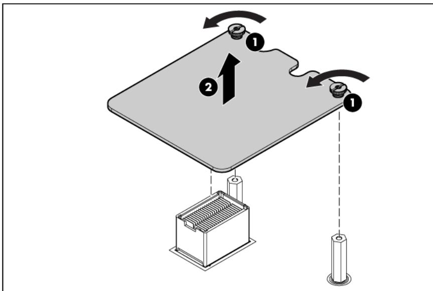
5. Locate the cache module ("System board components" on page 62).
