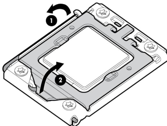
9. Using the processor tool, remove the processor from the system board:
