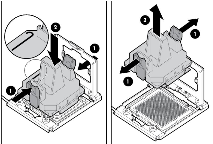
14. Carefully rotate the tool, and then push in and release the tabs to secure the processor in the tool.
