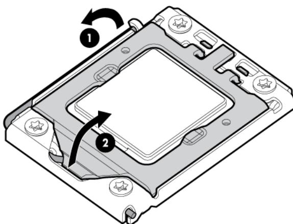
9. Using the processor tool, remove the processor from the system board:
