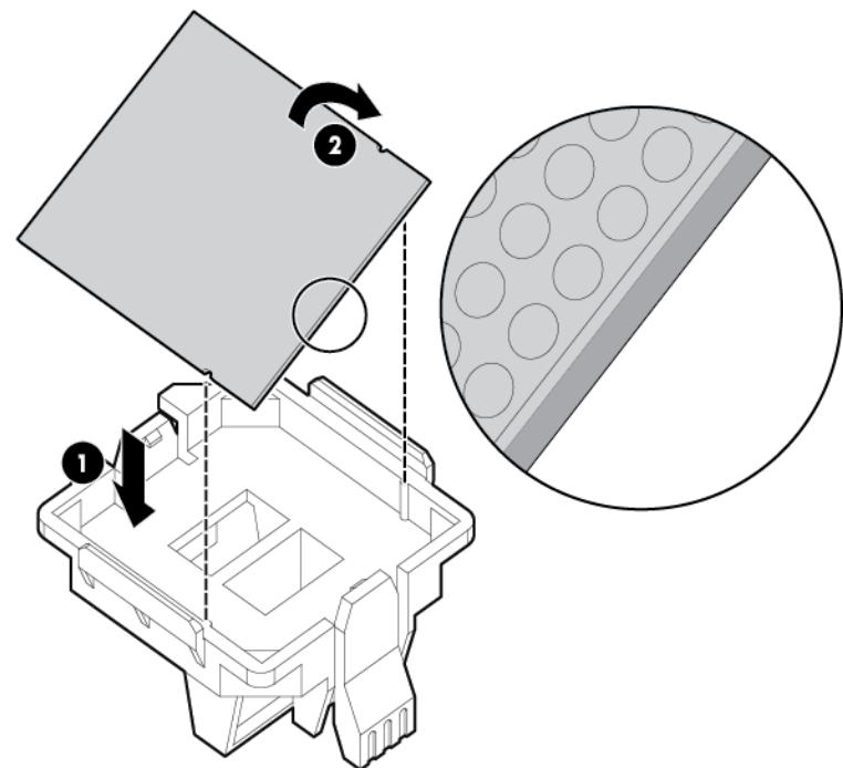
5. Align the processor installation tool with the socket, and then install the processor. **THE PINS ON THE SYSTEM BOARD ARE VERY FRAGILE AND EASILY DAMAGED.**
