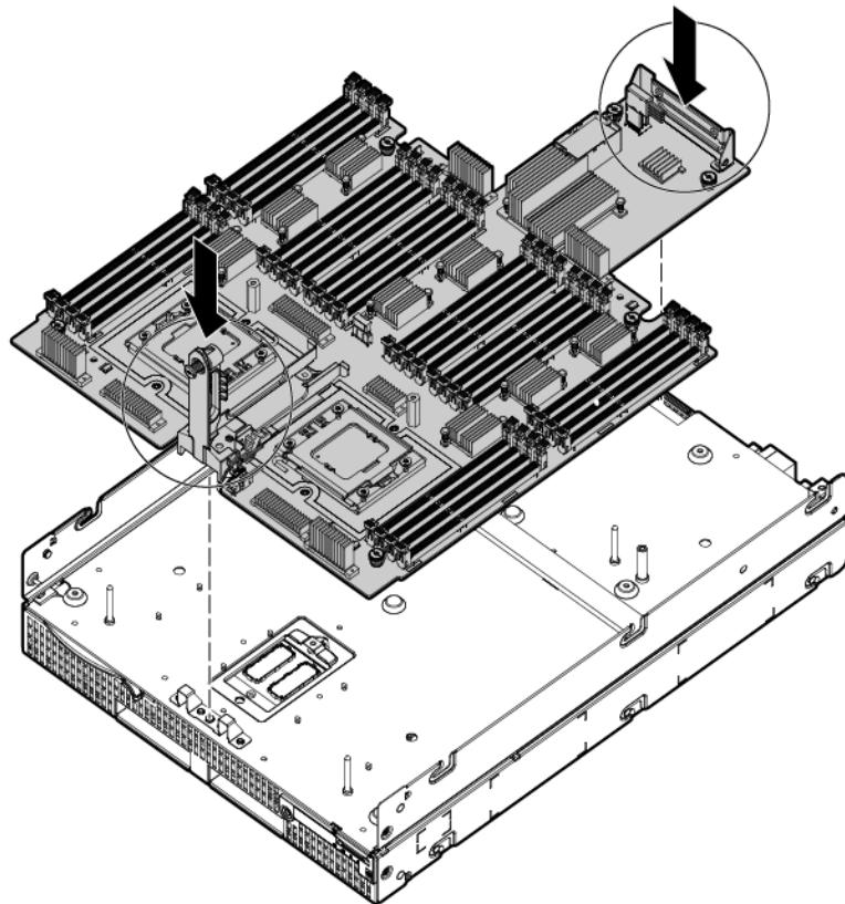
2. Lower the front handle, and then tighten the handle thumbscrew and the system board thumbscrews.
