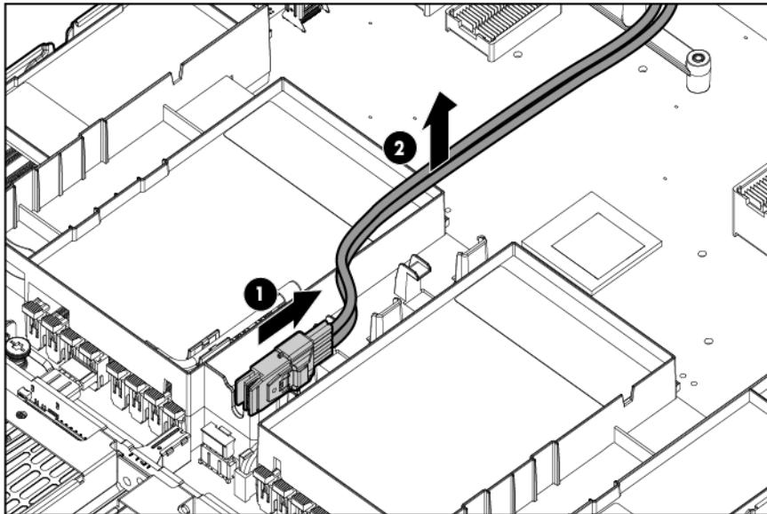
7. Remove the left DIMM baffle.
