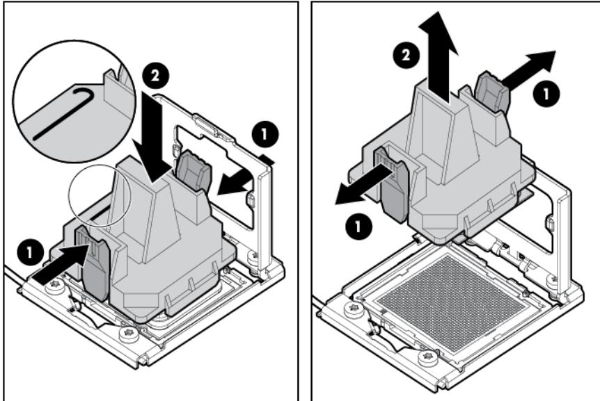
22. Carefully rotate the tool, and then push in and release the tabs to secure the processor in the tool.
