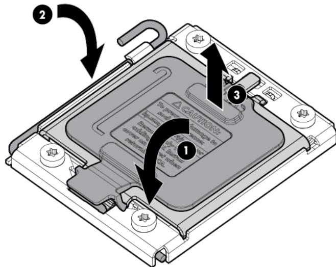
**CAUTION:** Be sure to close the processor socket retaining bracket before closing the processor locking lever. The lever should close without resistance. Forcing the lever closed can damage the processor and socket, requiring system board replacement.
