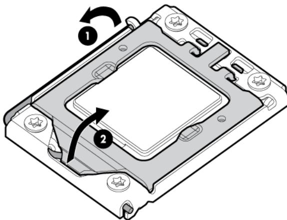
13. Using the processor tool, remove the processor from the system board:
