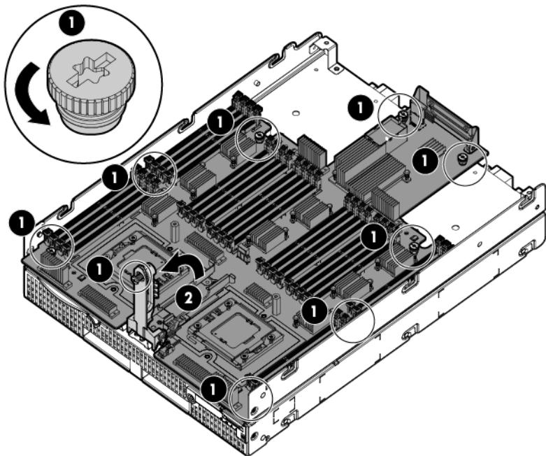
16. Using the front and rear handles, lift the failed system board from the server blade.
