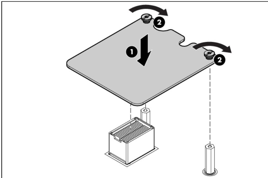
2. Install the access panel (A-side) ("Access panel (A-side)" on page 31).
