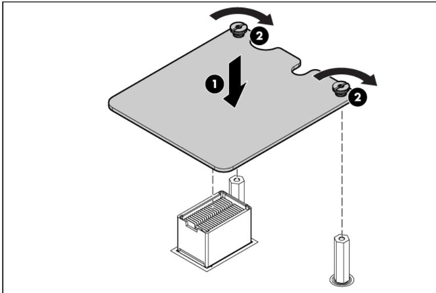
2. Install the interposer board ("[Interposer board](#)" on page [47](#)).
