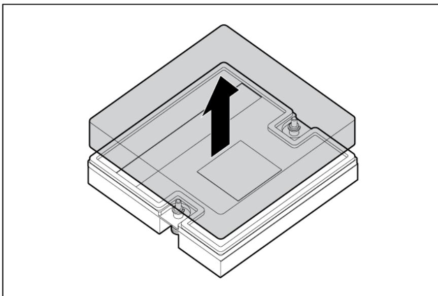
⚠ **CAUTION:** Orient the heatsink as indicated in the procedure. Otherwise, you cannot install the hard drive cage.
