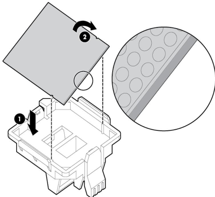
3. Align the processor installation tool with the socket, and then install the processor. **THE PINS ON THE SYSTEM BOARD ARE VERY FRAGILE AND EASILY DAMAGED.**
