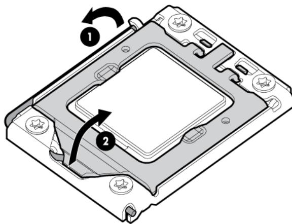
21. Using the processor tool, remove the processor from the system board:
