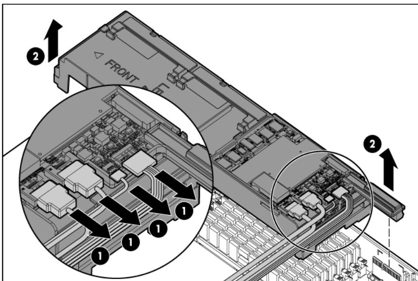
5. Remove the remaining DIMM baffle.
