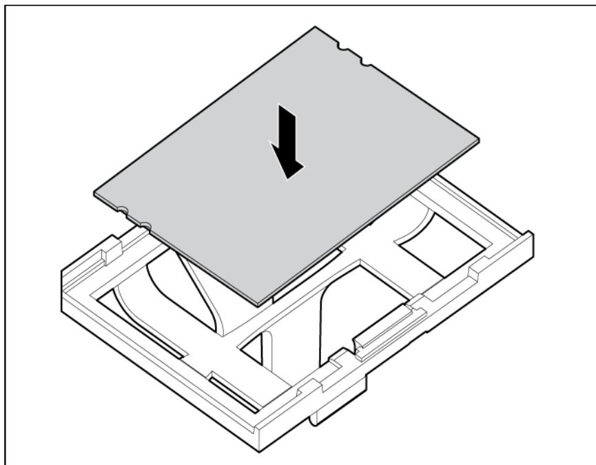
2. The processor fits one way into the socket. Use the alignment guides on the processor and socket to properly align the processor with the socket. Install the spare processor. **THE PINS ON THE SYSTEM BOARD ARE VERY FRAGILE AND EASILY DAMAGED.**
