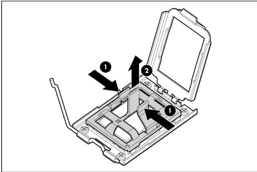
4. Close the processor socket retaining bracket and the processor locking lever.
