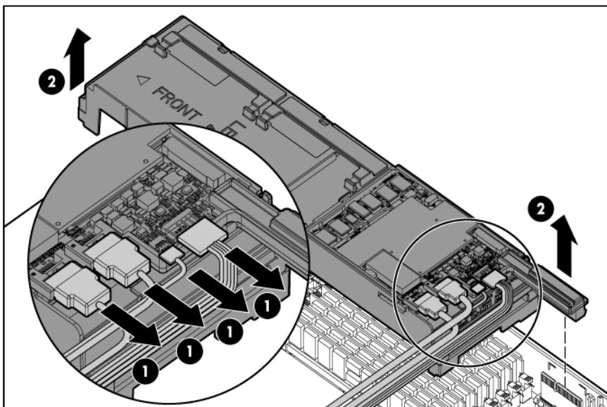
**5.** Remove the HP Smart Array Controller.
