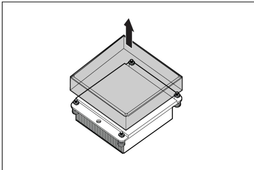
3. Align and install the heatsink. Alternate tightening the screws until the heatsink is seated properly.
