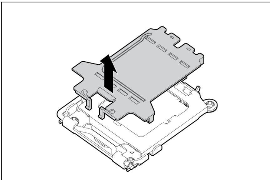
2. Install the processor socket cover onto the processor socket of the failed system board.
