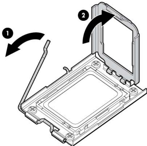
15. Using the processor tool, remove the processor from the system board.
