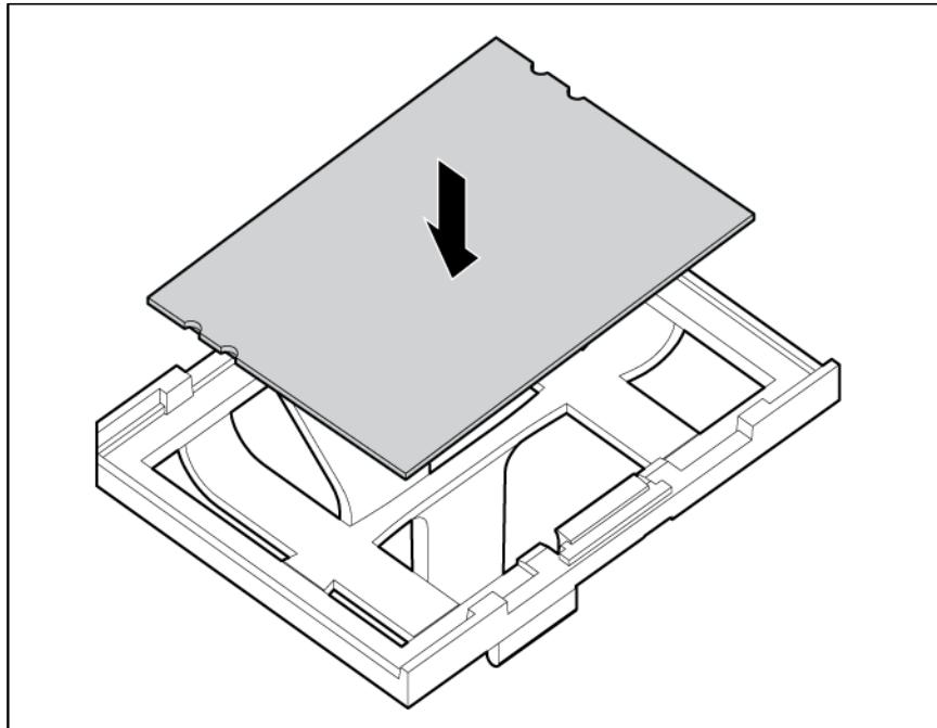
4. The processor fits one way into the socket. Use the alignment guides on the processor and socket to properly align the processor with the socket. Install the processor on the spare system board. **THE PINS ON THE SYSTEM BOARD ARE VERY FRAGILE AND EASILY DAMAGED.**
