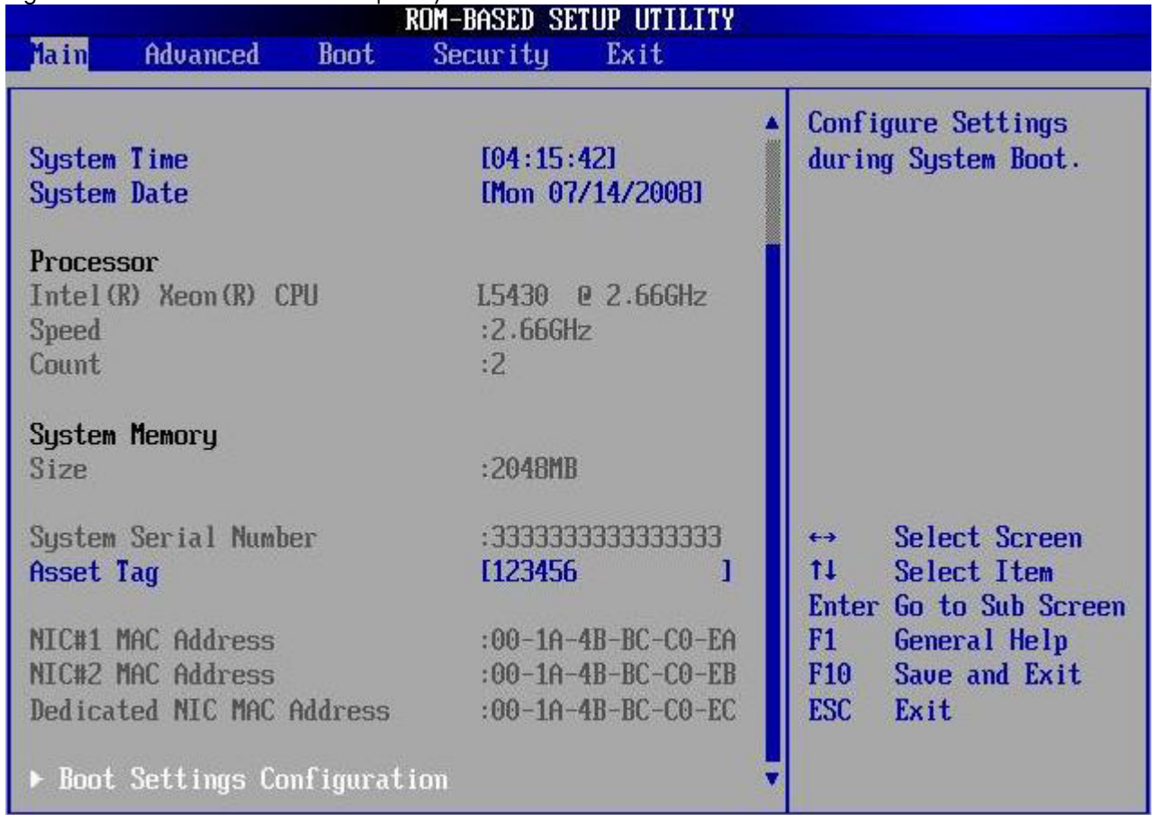
Figure 65 Main menu of the BIOS setup utility
