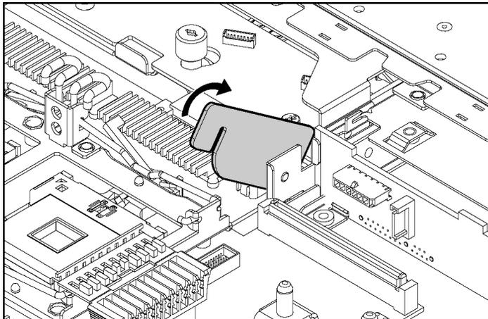
5. Release the processor retaining clips and processor locking lever.
