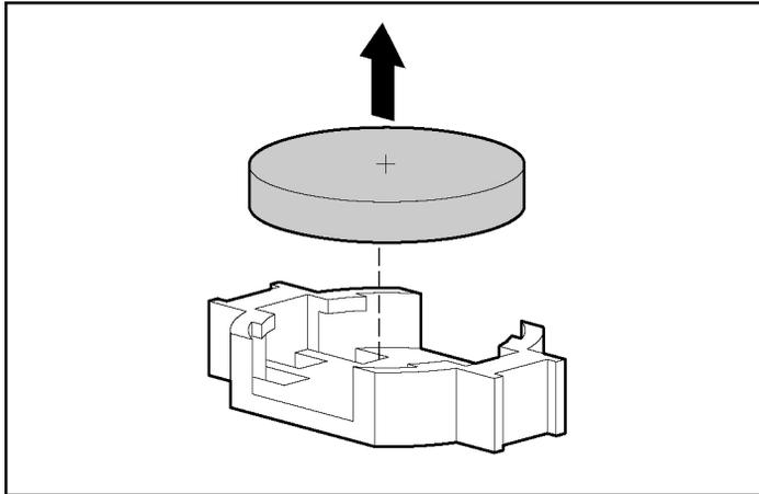
**IMPORTANT:** Replacing the system board battery resets the system ROM to its default configuration. After replacing the battery, reconfigure the system through RBSU.
