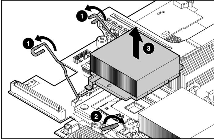
6. Lift the heatsink and processor from the server.
