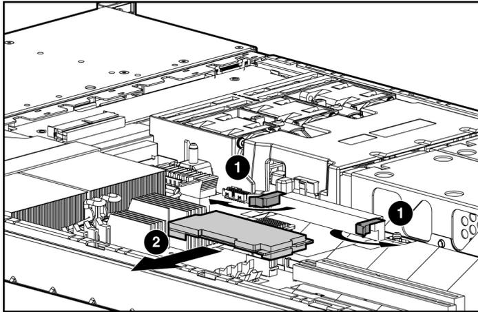
5. Remove the battery module cable from the cable clip on the system board.
