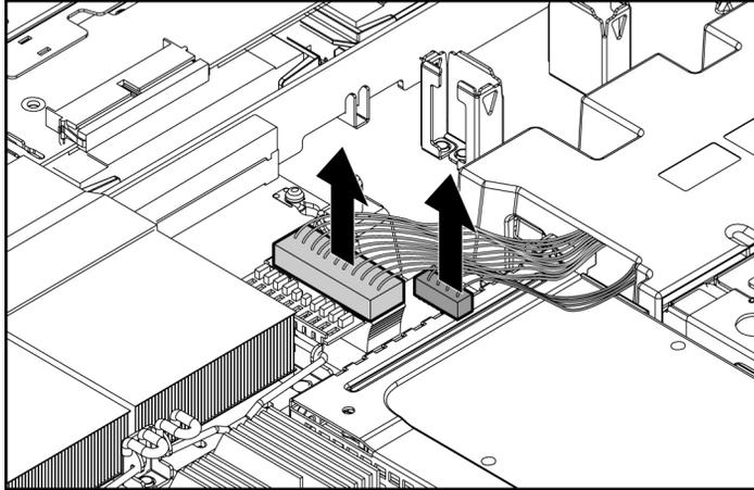
6. Remove the fan module ("Processor Fan Assembly" on page [29](#)).
