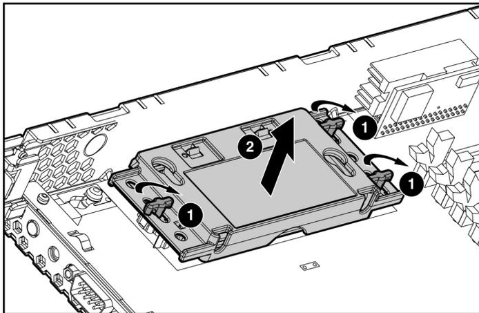
9. Remove the battery from the module.
