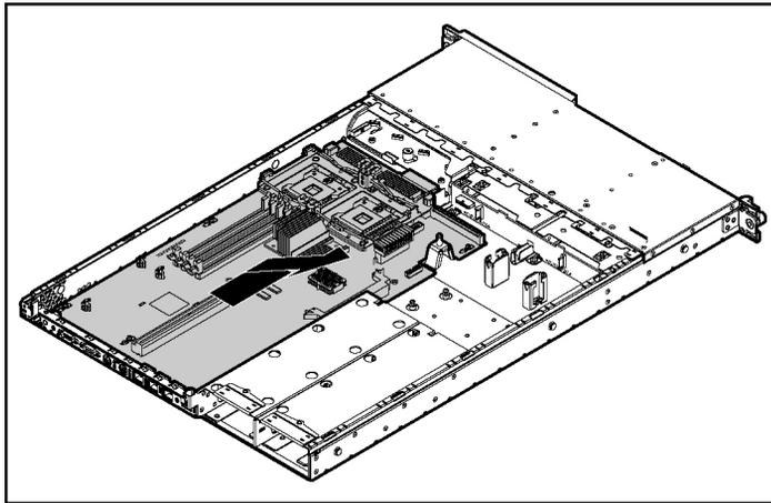
**IMPORTANT:** If replacing the system board or clearing NVRAM, you must re-enter the server serial number through RBSU.
