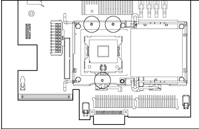
3. Install the processor and close the processor locking lever and processor retaining clips.
