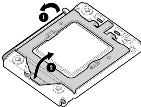
18. Using the processor tool, remove the processor from the system board:
