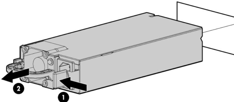
**WARNING:** To reduce the risk of electric shock or damage to the equipment, do not connect the power cord to the power supply until the power supply is installed.
