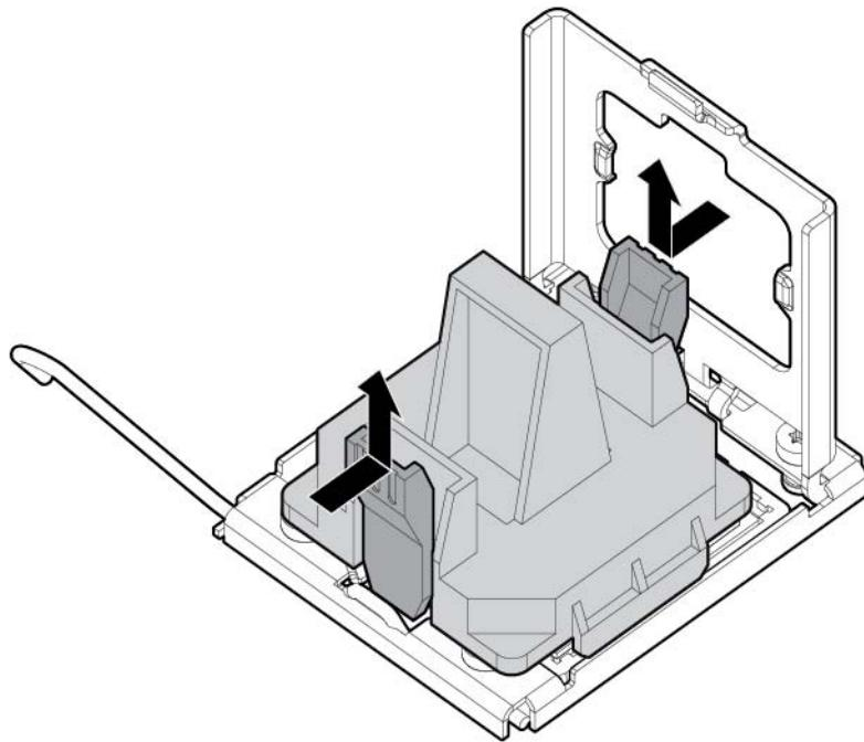
4. Close the processor socket retaining bracket and the processor locking lever.
