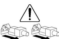
These symbols, on power supplies or systems, indicate that the equipment is supplied by multiple sources of power.
