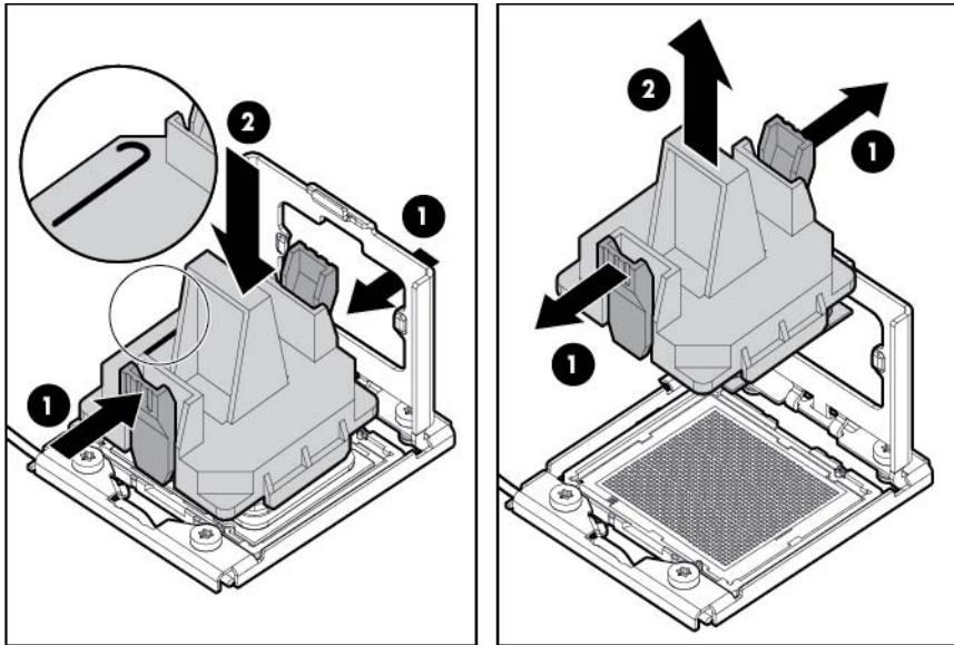
19. Carefully rotate the tool, and then push in and release the tabs to secure the processor in the tool.
