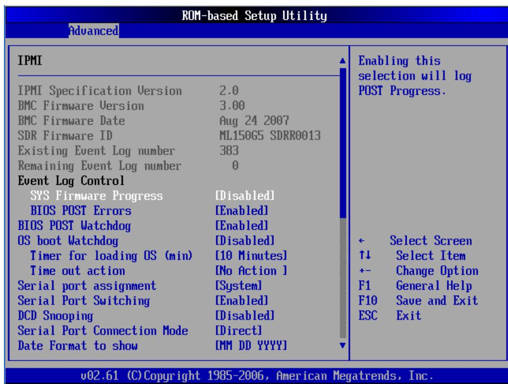
**Figure 4-9** Advanced menu—IPMI submenu, lower screen
