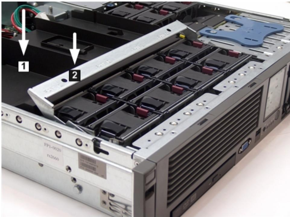
4. Ensure the fans have not become disconnected when opening the fan carrier handle by pushing down on all the fans to make sure they are seated properly.
