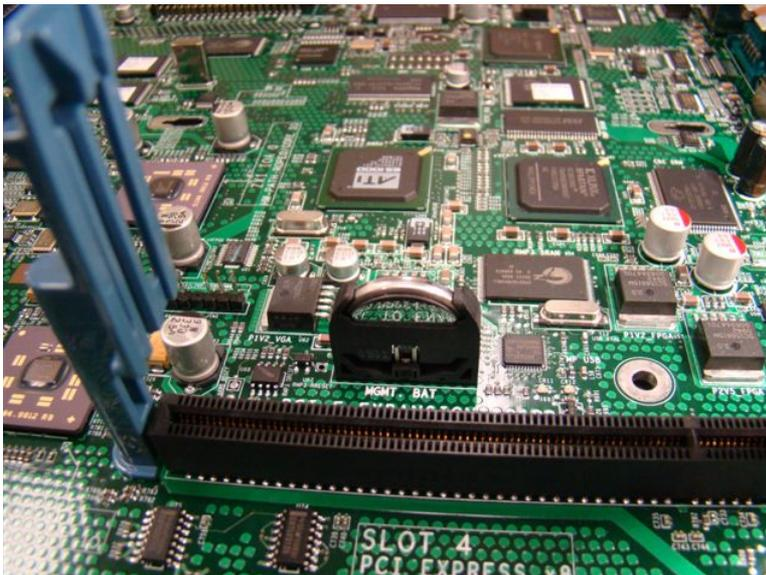
3. Ensure the battery is carefully removed. This is performed by holding the battery socket stationary with one hand while tilting the battery away from the battery socket using the other hand. See [Figure 77](#)
