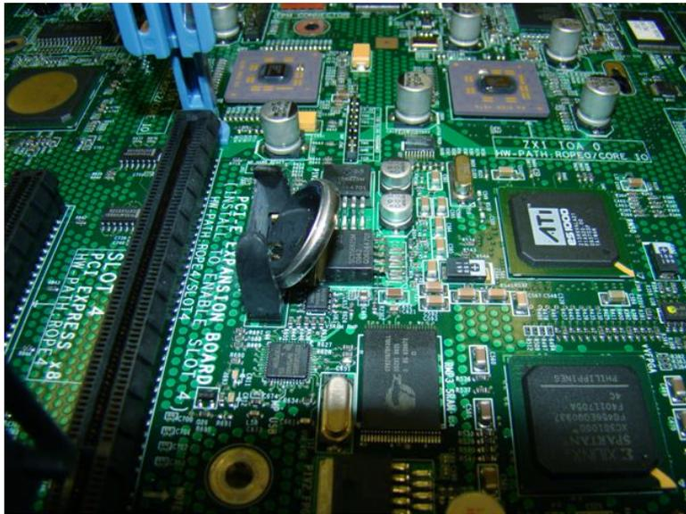
4. Use equal care when installing the new battery. Ensure the battery socket is stationary and cannot flex when installing the battery.
