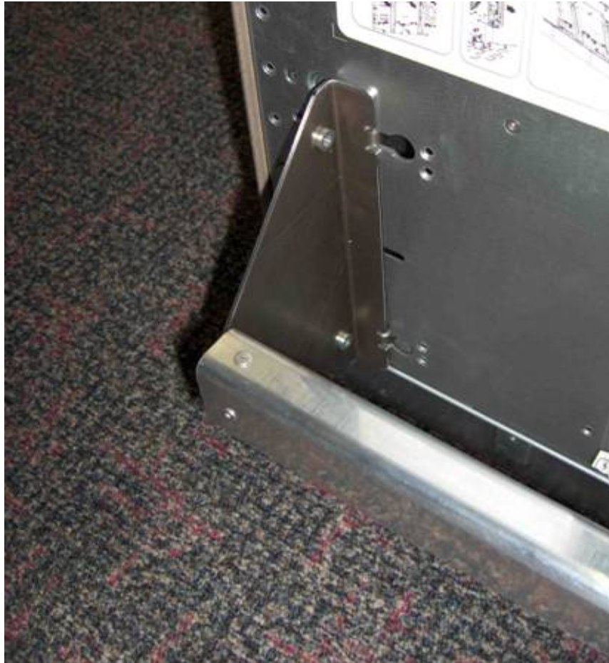
Figure 15 Inserting Rear Handle Tabs into Chassis
