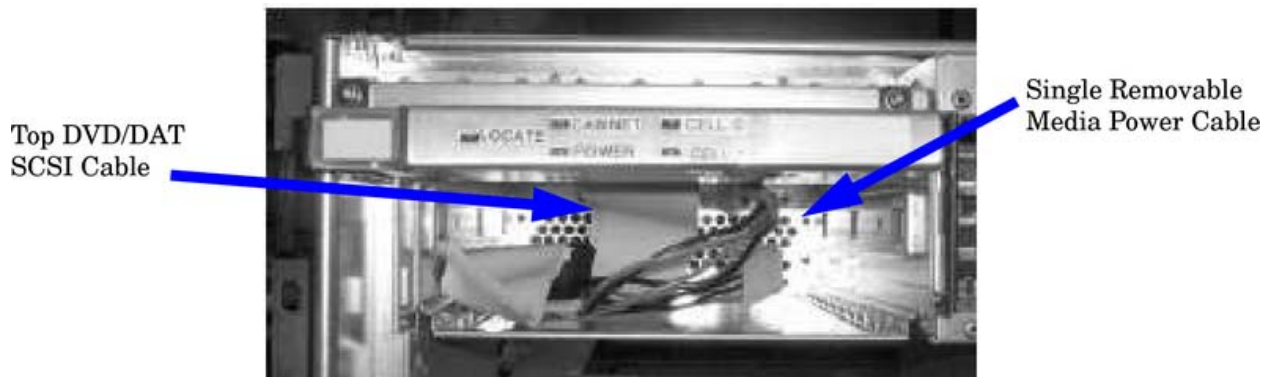
Figure 78 Single SCSI and Power Cable in Drive Bay
