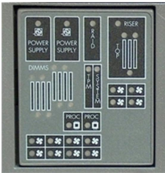
**NOTE:** The System Insight Display is the same for the Data Center server and the Office Friendly server. However, the Office Friendly server only uses the bottom row of fan LEDs since there are only six fans for the Office Friendly server.
